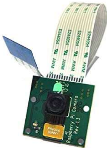
Figure 2. Raspberry pi camera 5mp
