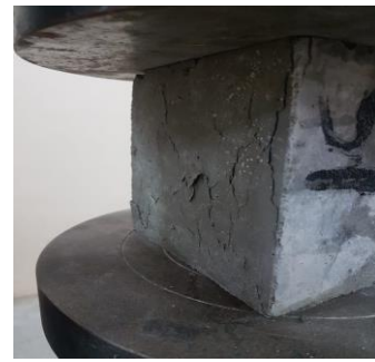
Fig.8 Failure of the specimen
