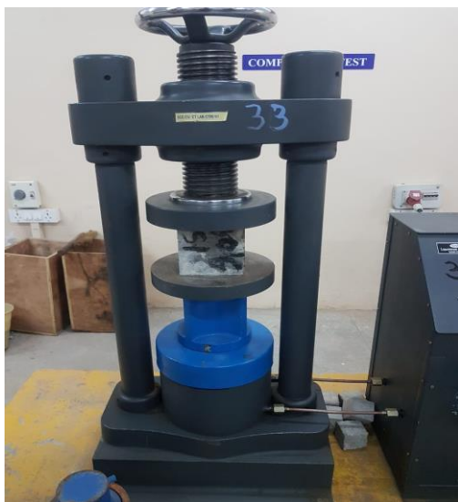
Fig.7 Compression test of cubes of size 150mmX150mmX150mm for 7 days
