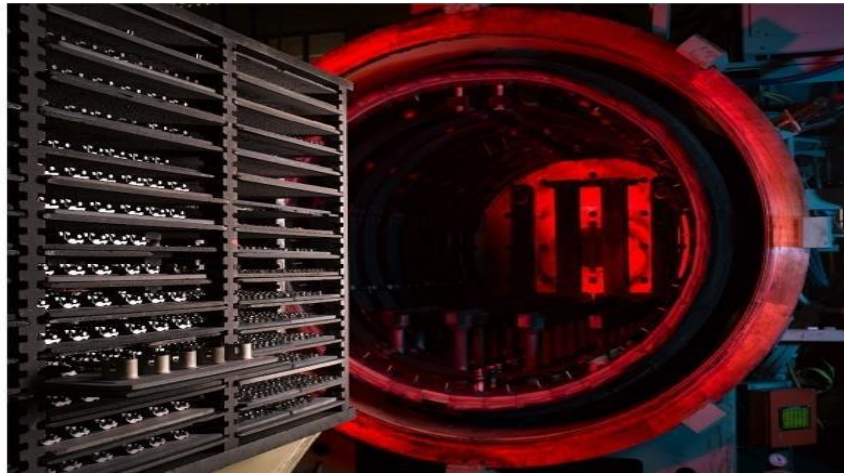
Figure 6: Batch type furnace
