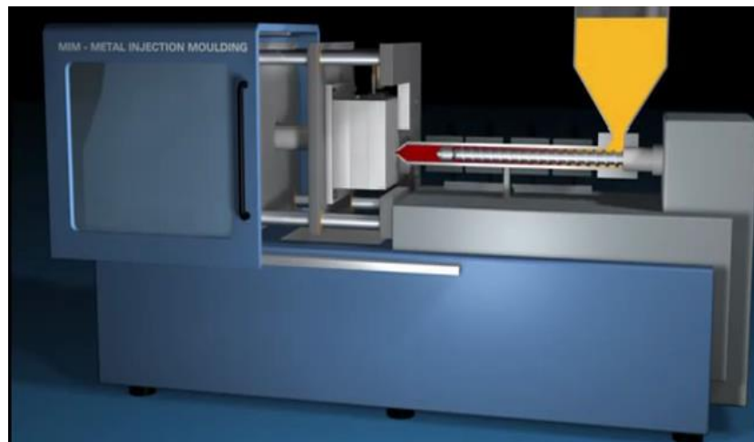
Figure 3: A typical injection molding Process
