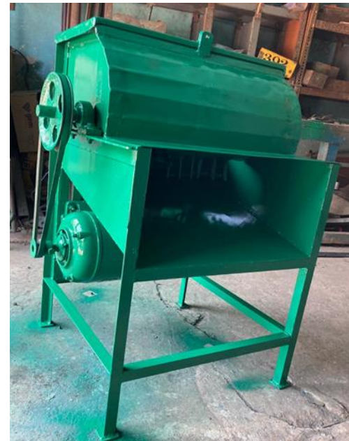
Figure.1: Groundnut Thresher Machine
