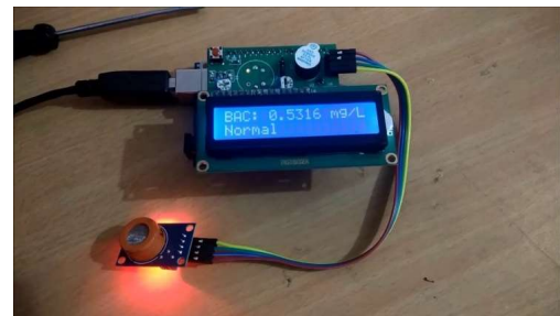
Fig.8 prototype working of alcohol sensor
