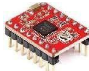
Fig. 7. A4988 Stepper motor driver module
