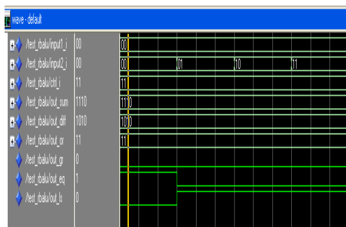
Figure 6 Simulated Result for Comparator Input1_i=-1 Input2_i=-1, 0, 1
