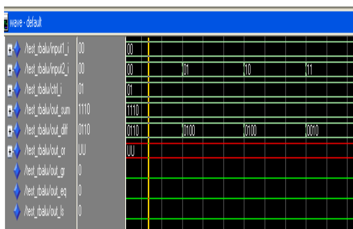
Figure 4 Simulated Result for subtractor Input1_i=-1 Input2_i=-1, 0, 1
