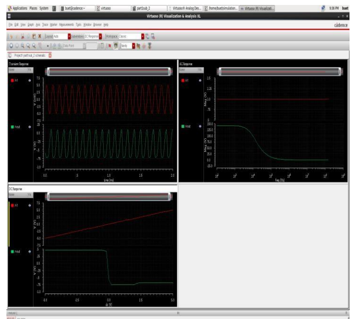
Fig 4. Op-amp circuit output using 90nm technology.
