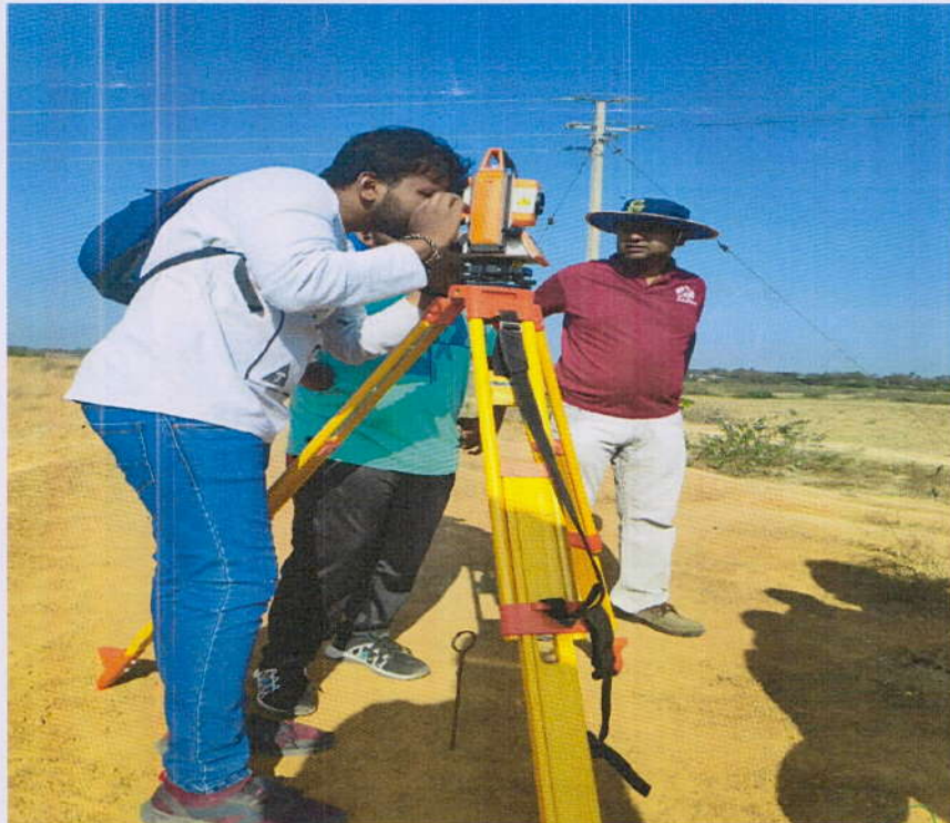
Tracing of capacity contour by using total station
